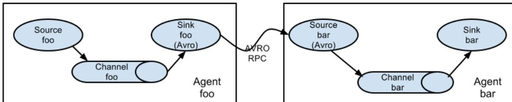
In order to flow the data across multiple agents or hops, the sink of the previous agent and source of the current hop need to be avro type with the sink pointing to the hostname (or IP address) and port of the source.
