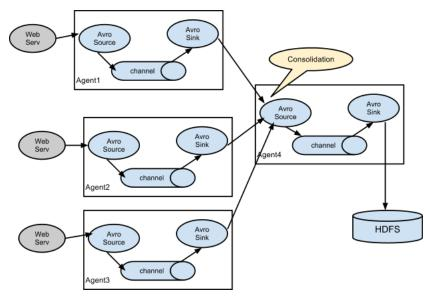
This can be achieved in Flume by configuring a number of first tier agents with an avro sink, all pointing to an avro source of single agent. This source on the second tier agent consolidates the received events into a single channel which is consumed by a sink to its final destination.
