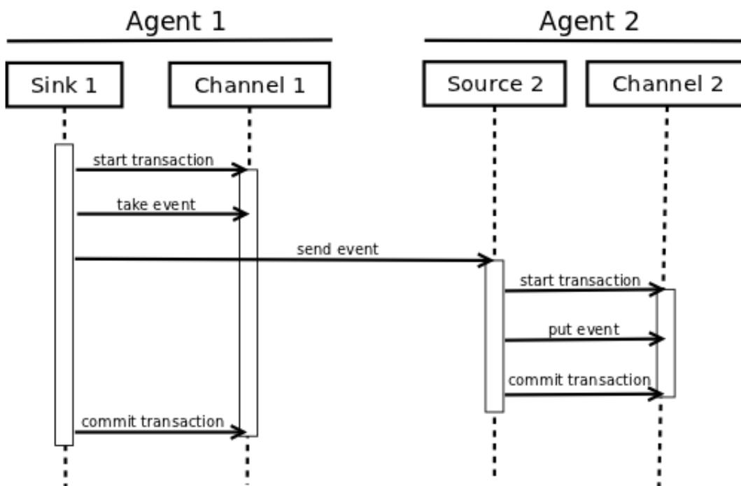
A `Transaction` is implemented within a `Channel` implementation. Each `Source` and `Sink` that is connected to `Channel` must obtain a `Transaction` object. The `Sources` actually use a `ChannelSelector` interface to encapsulate the `Transaction`. The operation to stage an `Event` (put it into a `Channel`) or extract an `Event` (take it out of a `Channel`) is done inside an active `Transaction`. For example:
